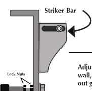
Adjusting the striker bracket is quick and easy. Drop the tailgate, close the lid down, and determine where the center of the latch will need to catch. The striker can easily move vertical and also forward/backwards. This must be done on every installation; Truck beds will vary slightly. Gaylords suggests monthly inspection of these parts to ensure perfect locking and unlocking for the duration of ownership.
